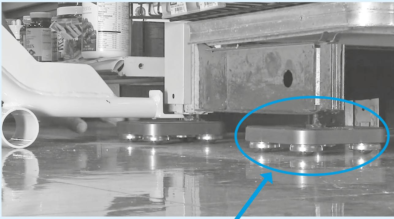
Reduced risk of tipping when load is lifted due to the low installation height profile
